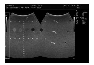
Closely spaced pin targets are ideal for testing high frequency transducers.
